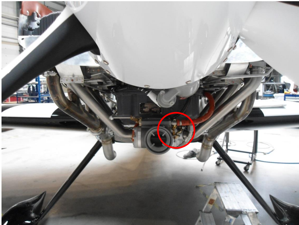
Figure 1: Location of the throttle control link.
