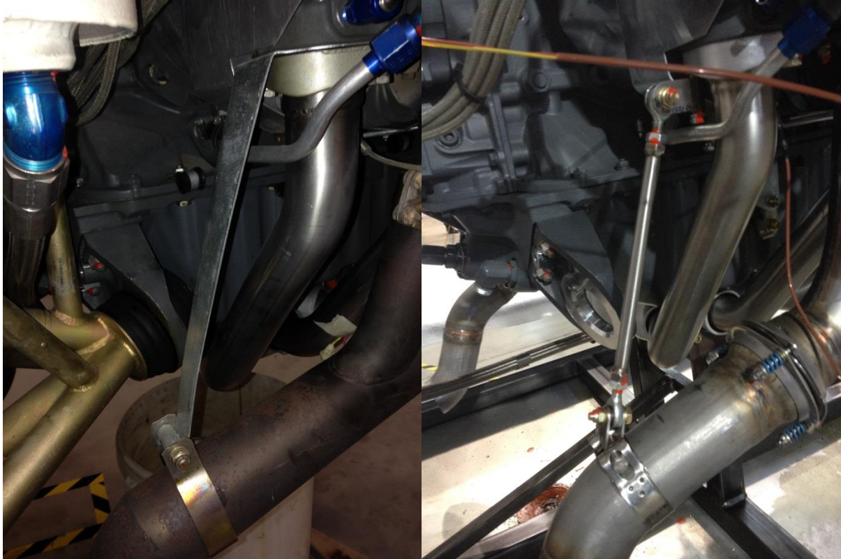
Figure 1: Old exhaust brace (XA42-7810-214) (Left); new exhaust brace (XA42-7810-101) (Right)
