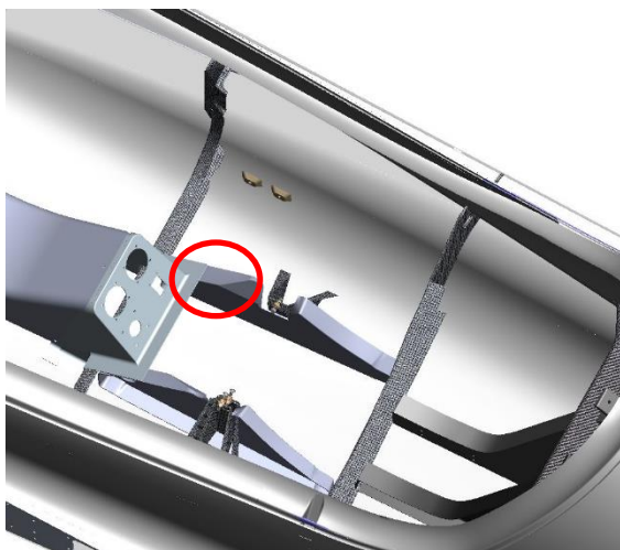
Figure 2: Position of the smoke relay, left: XA41 ; right: XA42
